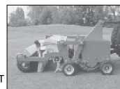
Wiedenmann®/ Terra-Combi® SHOWN W/SPIKED ROLLER & OPTIONAL OVERSEEDING UNIT
